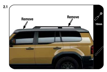
Remove the Factory Roof Rails and Saddle Brackets.
