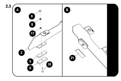
Assemble the 6mm and 10mm Spacers (Item 5 & 6) to the Front Foot Rail (Item 2) using a M6 x 30 Countersink bolt, M6 Flat Washer and M6 Nyloc Nut (Items 8, 10 & 17) as shown
