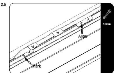
Place the Foot Rail in the ditch and align the slots of the mount with the OEM holes in the vehicle.
