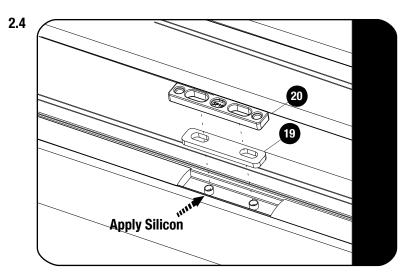
Apply a bead of silicon in and around each mounting hole.
