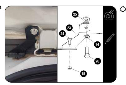
Loosen and remove the left side bolt of the Left Hand OEM Hinge to fit the Top Mounting Bracket (Item 23). This will act as a guide for the placement of the ladder.
