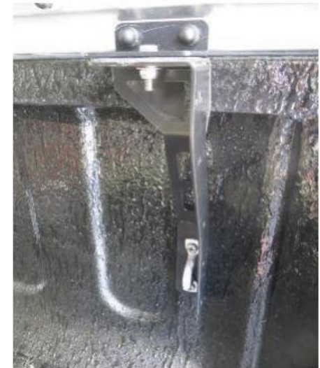
Figure 18.2: Rear-Right Support Bracket Installed
